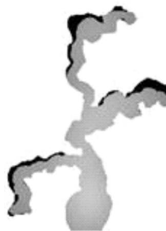
FIG. 3. Bowling chemical system. The picture shows the superposition of two pictures taken 2 s apart. This indicates the range of motion of the structure over the course of a single "bow."
